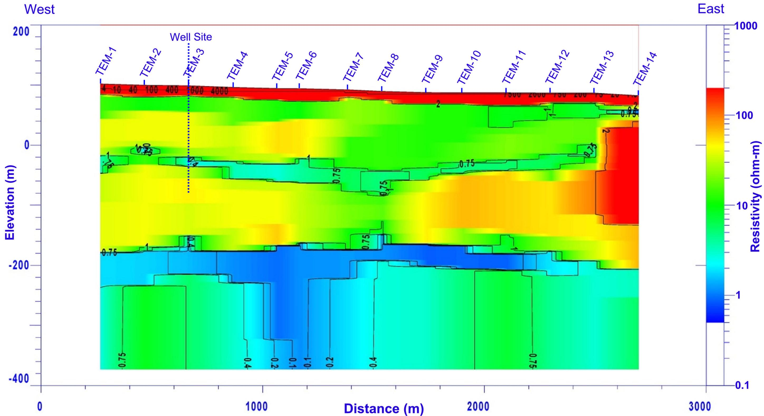
Resistivity Elevation Profile Generated by Program IX1D Developed by Interpex, Ltd.
