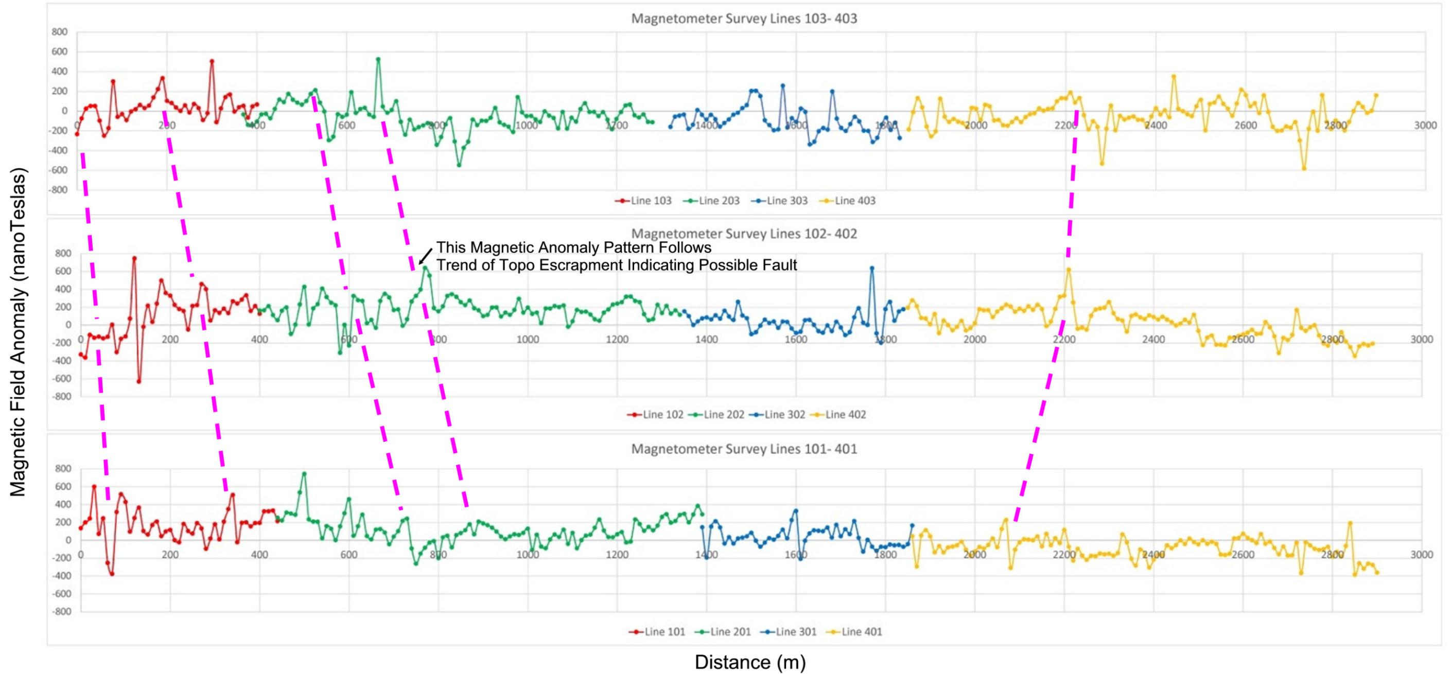
Dashed lines show interpretation of broader magnetic anomalies measured over intervals greater than 30 m. These anomaly trends could be caused by deeper subsurface structures such as faults in the basalt bedrock.
